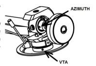
With the aid of a good magnifying glass adjust the needle until it is vertical in the groove (i.e. perpendicular to the record's surface). Ideally this should correspond to the top surface of the cartridge body being parallel to the record surface.
